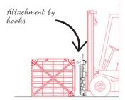
Forks up: single attachment by hooks for use with containers.
